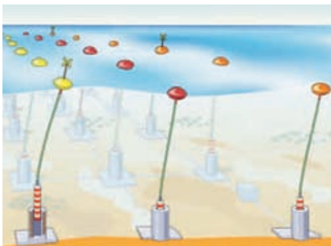
Seabased uses Pointabsorbers with a linear generator situated at the sea bottom
